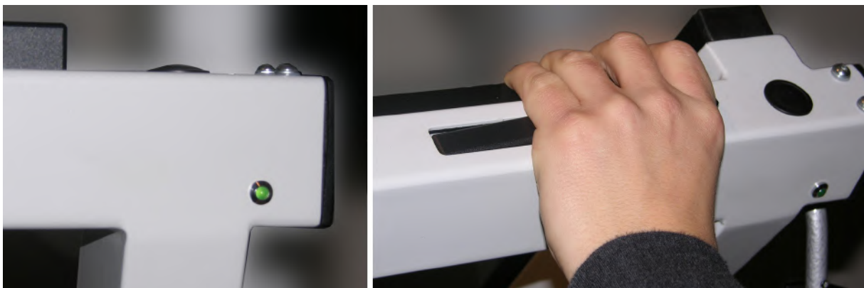
Illustration 6.7: left: Phoropter with green LED; right: Phoropter tilted, LED off
